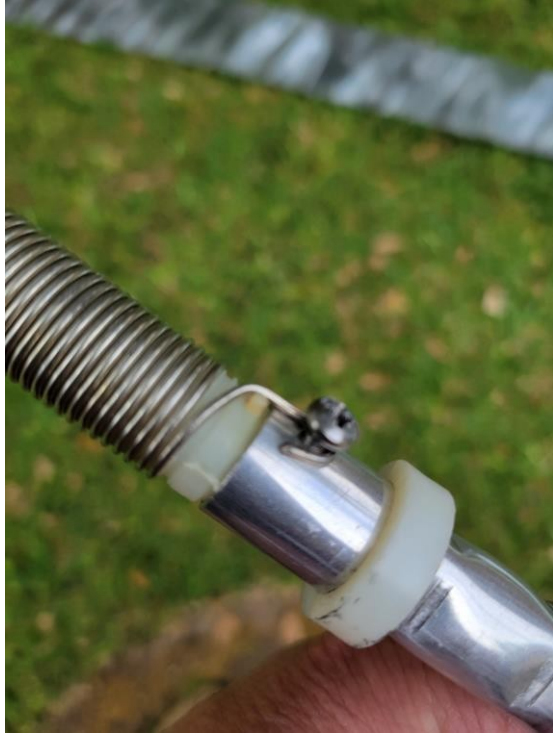
Figure 5 – Loose trap coil connection prior to tightening
