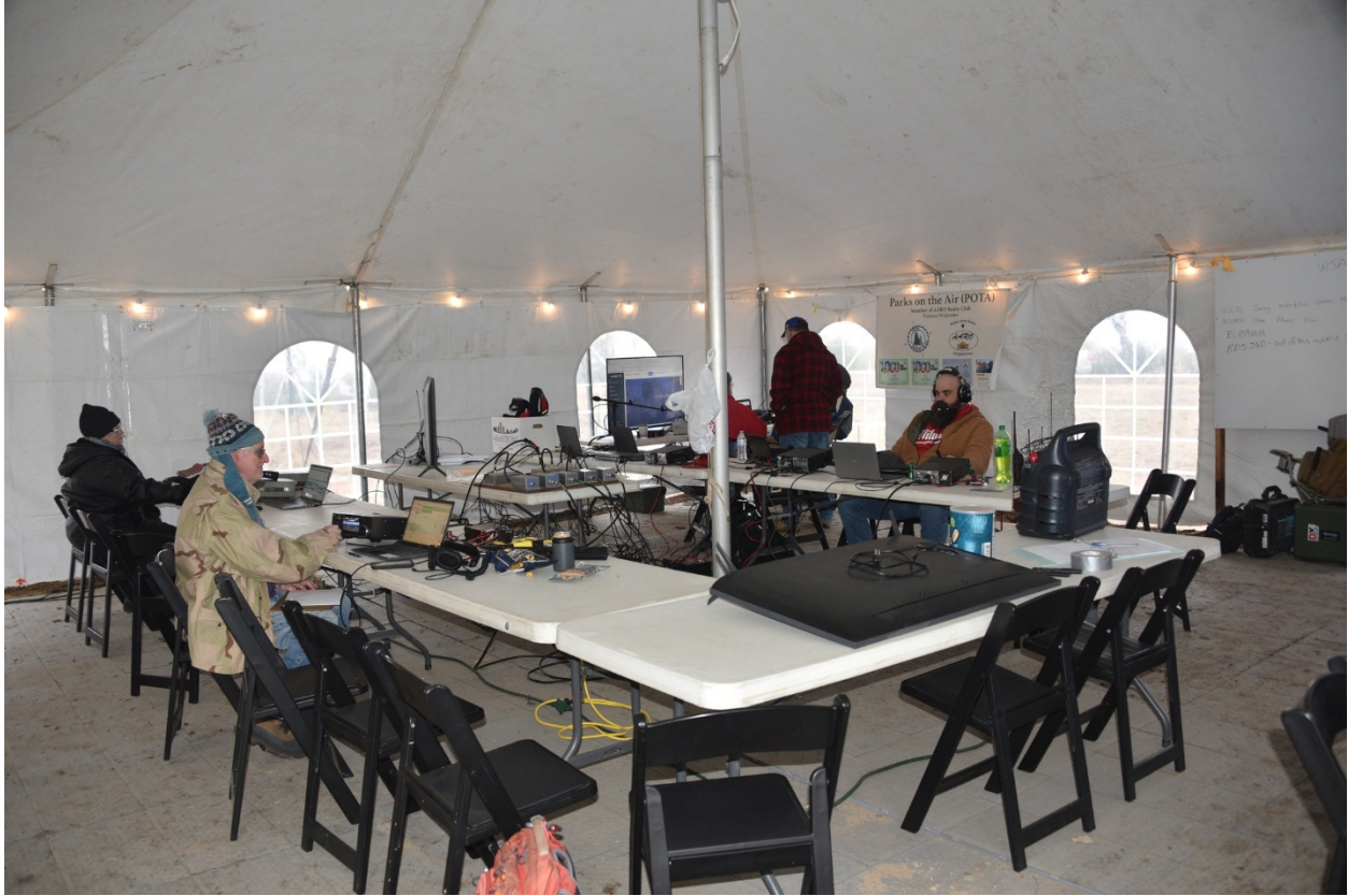
Inside the tent about noon on Saturday. The satellite station is in the right rear corner. Other stations are arranged around the U-shaped tables. The grey device in the center is a kind of multiplexer that allows different stations on different frequencies to use the same antenna, a vertical I believe. Only one connection per band. To switch bands, someone had to give up the appropriate antenna cable. It worked well. The black device on the corner of the table is a portable gas space heater. It was a very welcome item late at night.
