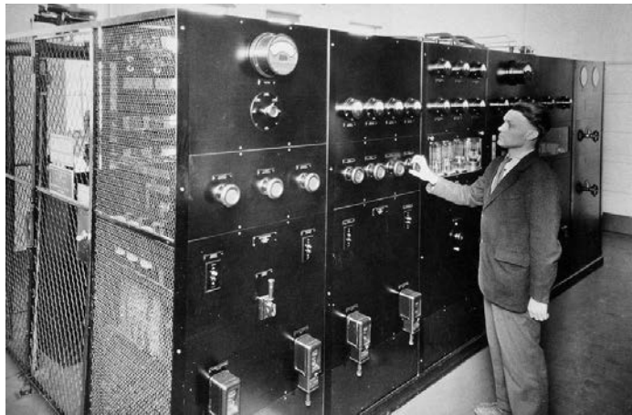
The WLW 5,000 watt WE 5C transmitter with operator Joe Whitehouse (from The Radio Historian)
