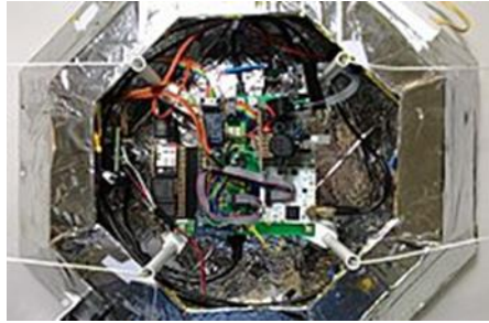
1Payload of an amateur high-altitude balloon for scientific purposes. Embedded computer Arietta G25, custom pcb and different sensors (temperature, pressure, passive radiation detector). Photo taken after the flight
