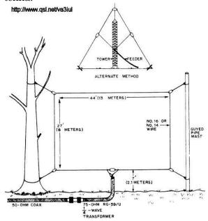
I used my antenna/tree system to hang the antenna. It is a small fiberglass bow, an arrow with a weighted tip and fishing line. The weighted arrow will fly almost straight up and down. With a number of trees available it was an easy task to get the antenna top up about 50 feet or so. The bottom was about 8 feet up as I recall. Dimensions are very approximate. I used a barrel to attach 52-ohm coax back to the shack in the basement of the house. I tweaked the antenna using a simple SWR meter.
